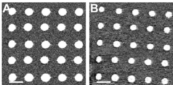
**Figure 5.** Electrochemical whittling of MHA nanostructures on Au(111) surface: (A) LFM image of an original MHA pattern on an Au(111) surface; (B) the same pattern in "A" after electrochemical whittling at  $-750$  mV for 2 min in 0.5 M aqueous KOH solution. The bar is 500 nm.
