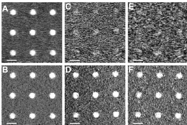
**Figure 9.** Topography (A, C, E) and LFM (B, D, F) images of a DPN-generated MHA dot array. (A, B) Original MHA array. (C, D) The same array in "A" and "B" after ODT passivation. (E, F) The same array in "C" and "D" after electrochemical desorption at  $-750$  mV for 5 min in KOH solution. The bar is 500 nm.
