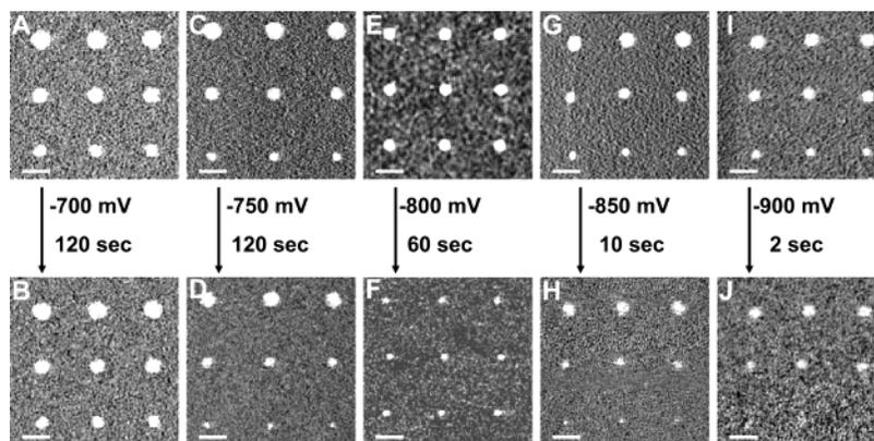
**Figure 1.** LFM images of DPN-generated MHA patterns before (upper) and after (below) electrochemical whittling at different potentials with different time lengths. The bar is 500 nm.
