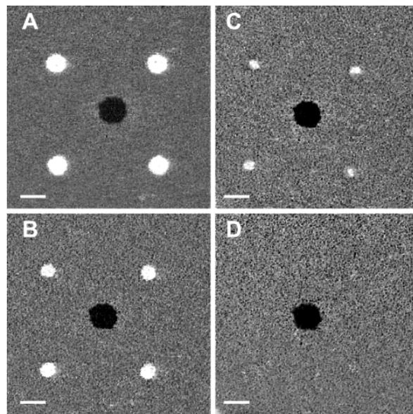
**Figure 11.** LFM images of ODT-MHA two-component array indicating selective whittling: (A)  $2 \times 2$  array of MHA dots (white) and an ODT dot (black); the array in "A" after applying a potential of  $-750$  mV for 3 min (B), 6 min (C), and 9 min (D), respectively. The bar is 500 nm.
