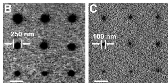
**Figure 7.** (A) Cyclic voltammogram for the reductive desorption of self-assembled monolayers of DODDSe on an Au substrate in 0.5 M aqueous KOH solution. The scan rate is 100 mV/s. (B, C) LFM images of a DPN-generated DODDSe pattern before (B) and after (C) electrochemical whittling at  $-450$  mV for 2 min in 0.5 M aqueous KOH solution. The bar is 500 nm.
