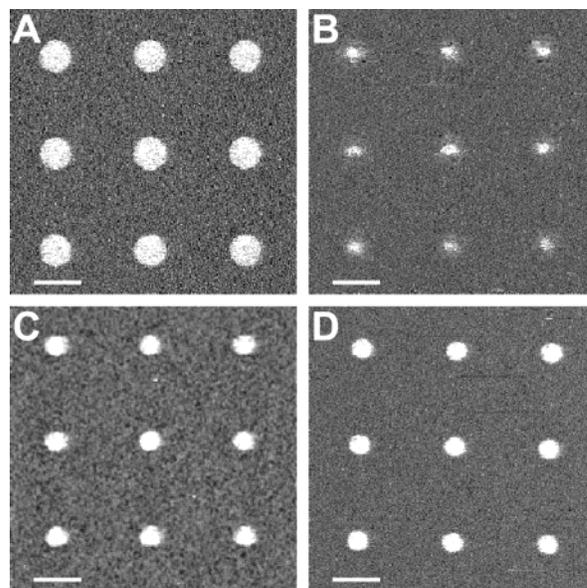
**Figure 4.** LFM images of MHA patterns: (A) 3 × 3 array; (B) the array in “A” after whittling at -1270 mV vs Fc/Fc<sup>+</sup> for 60 s in 0.1 M [CH<sub>3</sub>(CH<sub>2</sub>)<sub>3</sub>]<sub>4</sub>NBF<sub>4</sub> methylene chloride solution; (C) A 3 × 3 array; (D) the same array in “C” after whittling at -720 mV vs Fc/Fc<sup>+</sup> for 60 s in 0.1 M [CH<sub>3</sub>(CH<sub>2</sub>)<sub>3</sub>]<sub>4</sub>NBF<sub>4</sub> methylene chloride solution. The bar is 1 μm.
