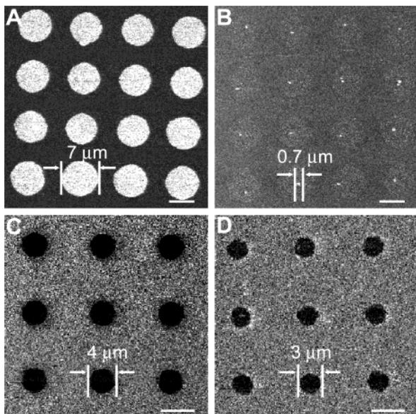
**Figure 8.** LFM images of  $\mu$ CP-generated patterns before and after electrochemical whittling. (A) Original MHA dots array. (B) The MHA dot array in the same area as in "A" after electrochemical whittling at a potential of  $-920$  mV for 30 s in 0.5 M KOH solution. (C) Original ODT dot array. (D) The ODT dot array in the same area as in "C" after electrochemical whittling at a potential of  $-1100$  mV for 5 min in 0.5 M KOH solution. The bar is 5  $\mu$ m.
