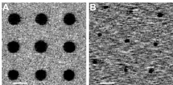
**Figure 6.** LFM images of a DPN-generated ODT pattern before (A) and after (B) electrochemical whittling at  $-1000$  mV for 5 min in 0.5 M aqueous KOH solution. The bar is 1  $\mu\text{m}$ .
