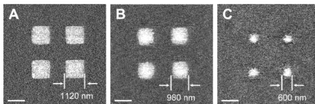
**Figure 10.** LFM images of DPN-generated MHA squares on a polycrystalline gold surface before and after electrochemical whittling: (A) original MHA squares; (B) the same MHA pattern as in "A" after electrochemical whittling in 0.5 M KOH solution at a potential of  $-750$  mV for 3 min; (C) The same MHA pattern as in "B" after electrochemical whittling in 0.5 M KOH solution at a potential of  $-750$  mV for another 7 min. The bar is 1  $\mu$ m.
