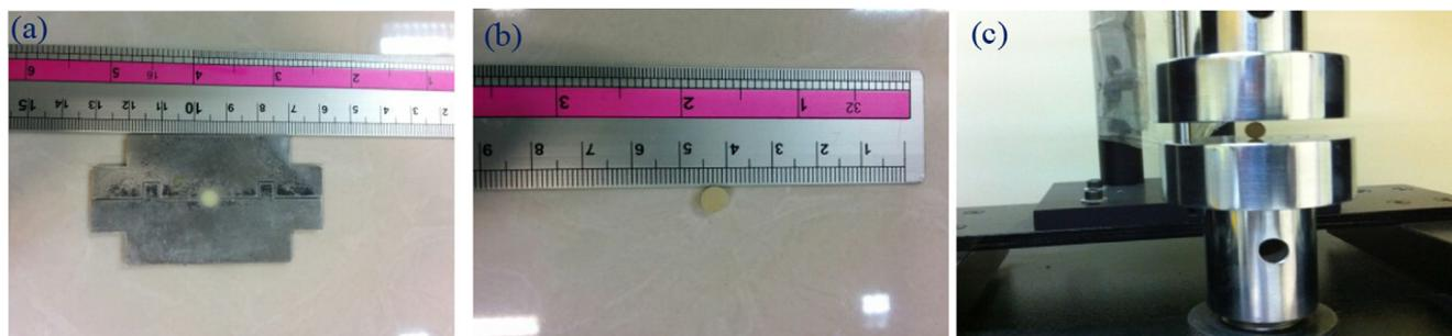
Fig. 5. (a) mold for resin casting, (b) prepared sample, and (c) test instrument.
