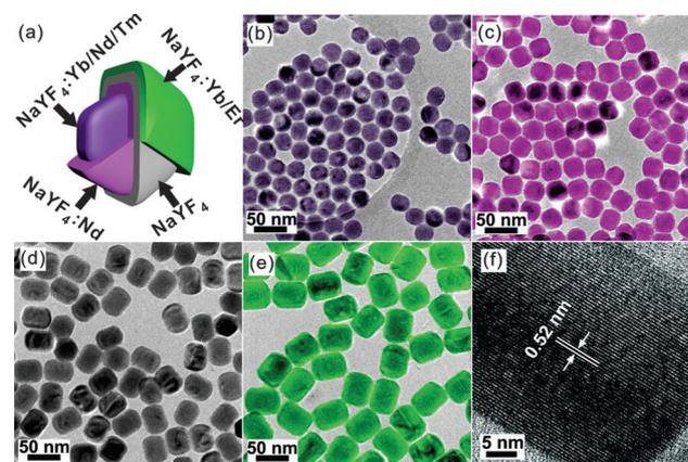
**Figure 1.** a) Composition of each layer of Tm@Er UCNPs. The false color of each layer represents the corresponding nanoparticles shown in (b–e). b–e) Low-resolution TEM images of Tm@Er UCNPs constructed by epitaxial layer by layer growth. f) High-resolution TEM characterization of a single Tm@Er UCNP. The lattice extending across the particle without interruption is indicative of its monocrystalline structure.
