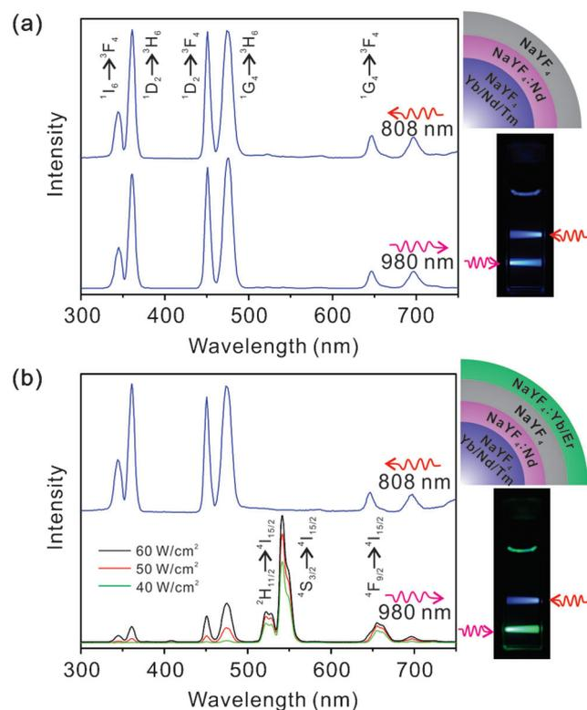
**Figure 2.** a) Upconversion luminescence profiles of the luminescent core with photon-inert shell and b) the Tm@Er UCNP under different wavelength excitations and varying power densities. The structures of the corresponding nanoparticles are illustrated in the right panel. The photographs show the UCNP in hexane solution (1 wt%) under irradiation by two laser beams at wavelengths of 808 nm and 980 nm. The power density for 808 nm and 980 nm lasers is 60 W cm<sup>-2</sup>.
